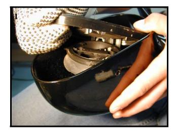
While using sturdy gloves, position your fingers behind the outboard edge of the mirror. Pull back on the mirror to dislodge it from the center hub and remove the mirror from the housing.
